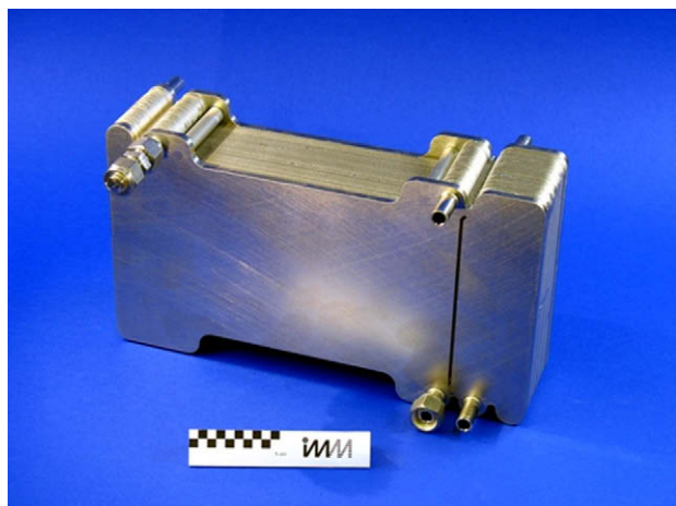
Figure 5. Microstructured pilot reactor for the MCE synthesis for operation up to 160 bar and 250 °C.
